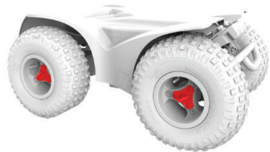
Figure 5.2d Extreme X8 lifting points (sold separately)
