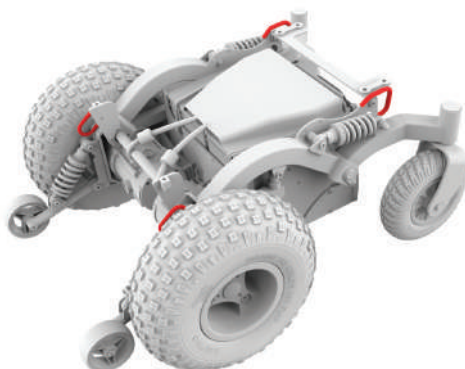
Figure 5.4c Frontier V4 tie downs
