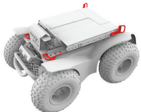
Figure 5.4d Extreme X8 tie downs
